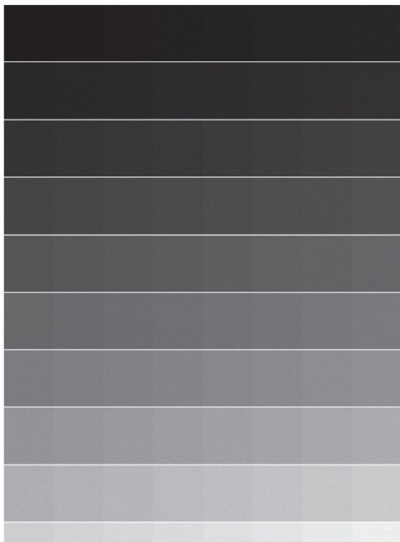
Fig. 2 A digital chart with 80 steps that changes by pixel value 50 between 145 and 4095 was used in order to control the highest optical density and linearity of the laser imager.
