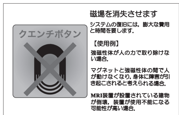
Fig.7 The display of the criteria. By displaying the function and the criteria of the button, it becomes useful under emergency situation.
