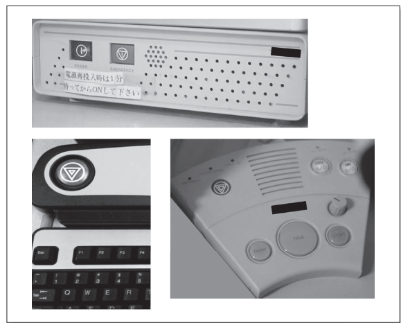
Fig.2 Emergency stop button The location of an emergency button is different among the manufactures. The actual color is red, and the design is similar.
